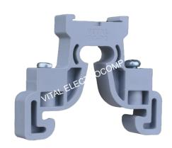
Vital make EC-P2 end clamp is designed to fit on a 35 mm din rail. The clamp can be slid on the rail and then tightened with screws to tightly secure the terminals on the rail from the end.
